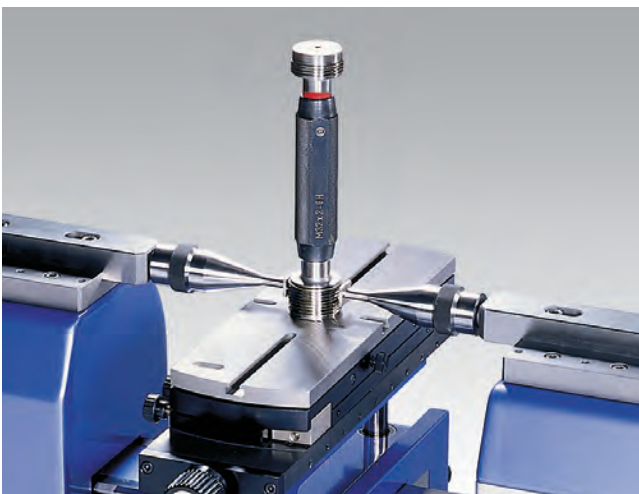
▲ Setting of threaded plug gages from diameter 1.18" to 9.84" (30 to 250mm) using table (54-196-160-0), small \varnothing anvils (54-190-806-0) and thread wires (54-197-007-0)
