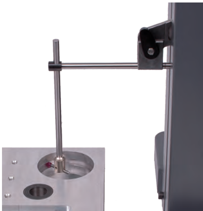
Internal groove measurements with accessories 54-199-508, 54-199-506 and 54-199-501
