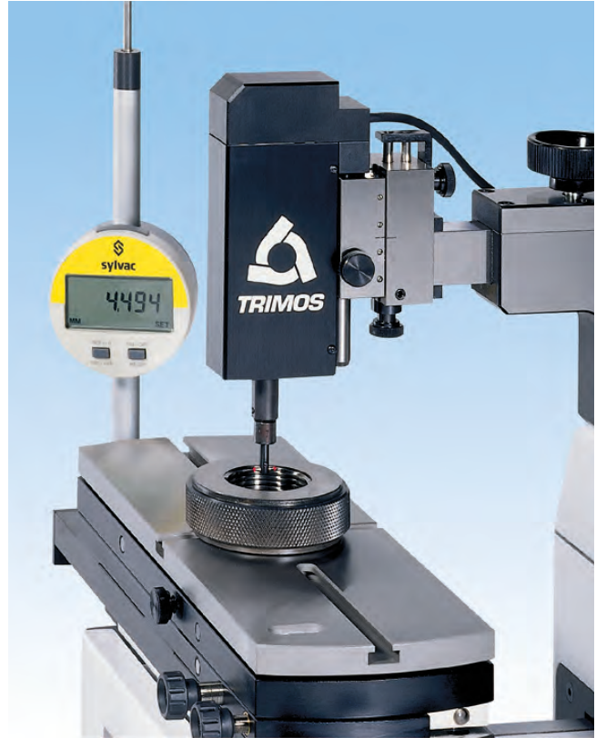
▲ Checking of threaded ring gages from pitch 0.7 to 6mm/48 to 4 threads per inch (max. internal dia. 7.08"/180mm) using table (54-197-011-0), clamps (54-197-142-0), Internal measuring device (54-197-074-0) & T-Ball probes (54-197-075-0)
