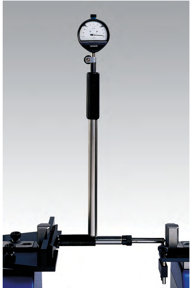
▲ Setting of 2-point bore gages using gage block anvils (54-190-805-0), bore gage centering supports (54-190-829-0) and secondary contact support (54-196-040-0)
