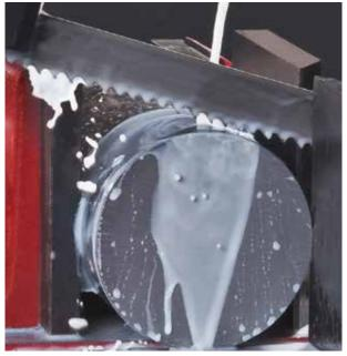
Start to cut material at reduced cutting rate
