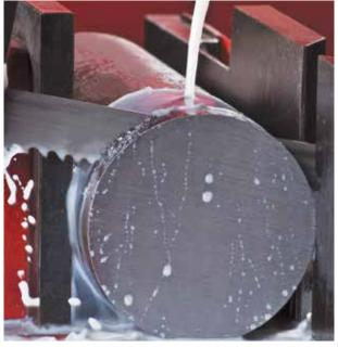
After break-in when the blade has fully entered the work-piece, increase the feed rate over a series of cuts until the recommended cutting rate is achieved
