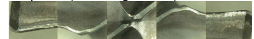
Competitor A (Total Drilling 470 Holes)
