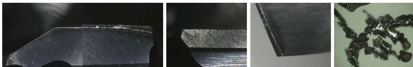
COMPETITOR B (Total Drilling 400 Holes)
