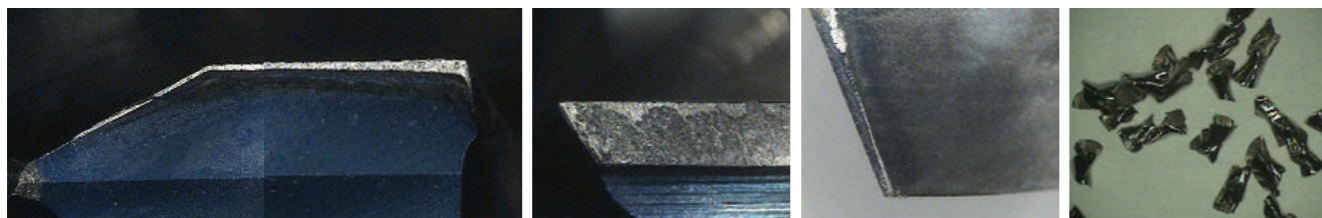
COMPETITOR B (Total Drilling 400 Holes)
