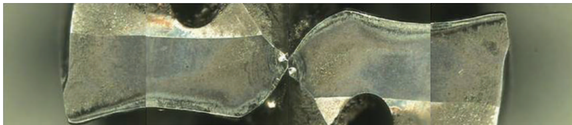
YG-1 (After Drilling 1,000 Holes)
