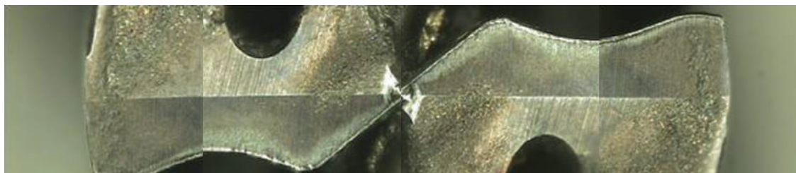
COMPETITOR A (After Drilling 546 Holes)
