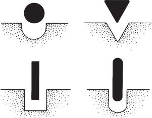
A flat file should be used for general-purpose work, a square file for enlarging rectangular holes and a round file for enlarging round holes. A half-round file can be used for dual purposes, the flat face for filing flat surfaces and the curved face for grooves.
