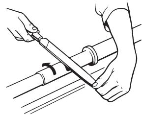
Lathe filing is usually employed for fitting shafts. Where stock is to be removed, a 12"/300mm or 14"/350mm Long Angle Lathe file is preferable. This file will provide the finish suitable for a drive fit. For a running fit a Mill file will provide a smooth finish. Where
