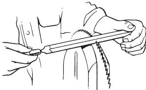
rakers clear the cut. This is filed at an angle of 45° from the filer. This permits access to cutters and enables the teeth to be filed at the correct angle.
