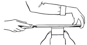
file; the tip of the thumb pointed forward. For lighter strokes however, the thumb can be turned to as much as right angles to the direction of the stroke
