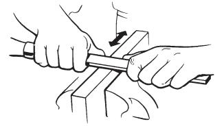
Normally, a standard Mill Bastard file is used for drawfiling, but where a considerable amount of stock has to be removed, a Flat or Hand file (Double Cut) will work faster. However, this roughing down leaves small ridges that will have to be smoothed by finishing with a Single Cut Mill file.
