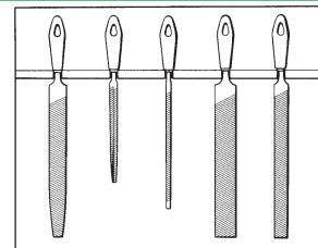
The file teeth should be kept clean at all times by using a file card, or a wire file brush, to clear the grooves between the teeth.
