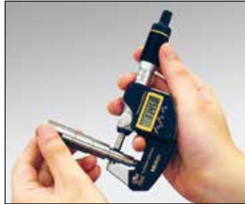
Measuring coaxial workpiece
