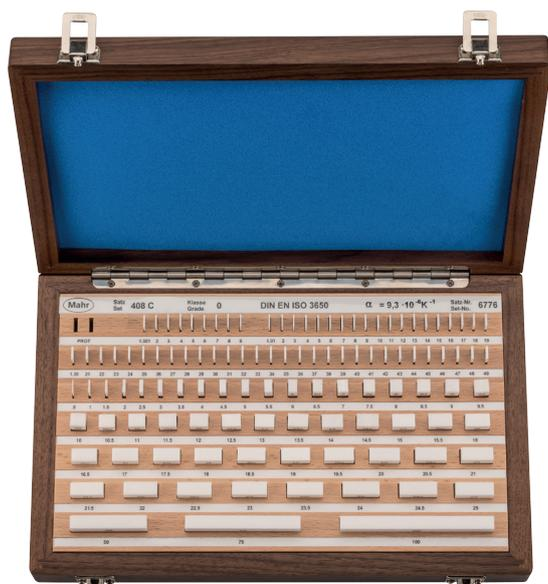
Resistant to both impact and breakage. Virtually no warping of material if surfaces become scratched or edges damaged. Longer retention of wringing ability
