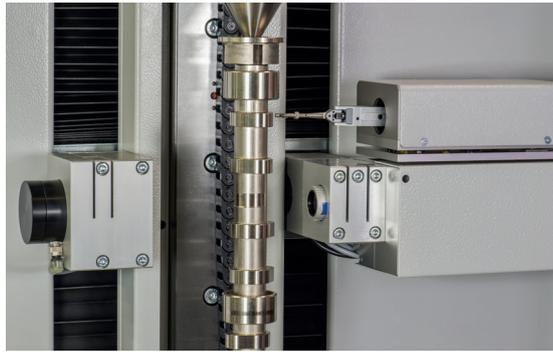
Tactile measuring unit with y-measuring axis 60 mm
