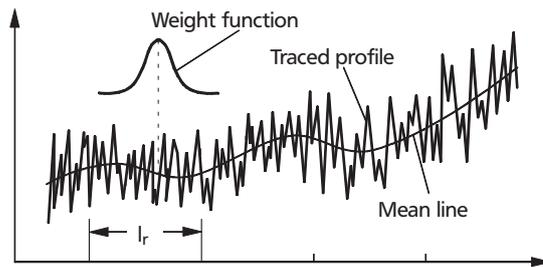
**Profil filters** separate into long wave and short wave components. The  $\lambda_c$  profile filter separates the roughness profile from long wave components (e. g. waviness). **R-profile** (roughness profile) represents the deviations of the primary profile from the mean line of the  $\lambda_c$  profile filter. When presenting the roughness profile, the mean line is the zero line.
