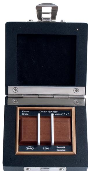
Resistant to both impact and breakage. Virtually no warping of material if surfaces become scratched or edges damaged. Longer retention of wringing ability
