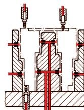
Measurement of hole distances of truncated cylindrical bores with jet air plug gages measurement as per the differential measuring method.
