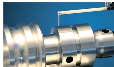
BFW probe system with magnetic probe arm holder
