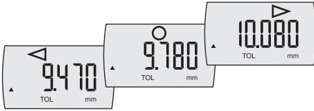
**Tolerance indication without the value in the display.** In and out of tolerance will be indicated in the display as a symbol.
