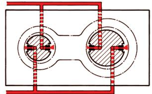
Mating measurement between bore and shaft with jet air plug gage and jet air ring gage.
