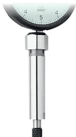
For extending reach of all ANSI/ AGD type and perpendicular indicators with .375" diameter stems and ranges up to 6.35 mm/ .250" range. Attaches to indicator stem by integral split collet. Body is 12 mm/ .500" OD.
