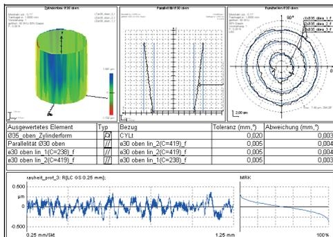
MarForm MMQ 400 is suitable for universal use for extensive workpiece evaluation according to DIN ISO 1101.
