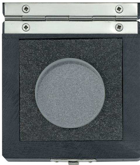
Used to test the surface flatness on precision components or measuring instruments according to the interference principle
