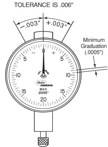
*Your tolerance spread is .006". You have chosen an ANSI/AGD Group 2 (Mahr "C" Size) dial with a minimum graduation value of .0005". Mahr offers four indicator types in this size and minimum graduation value. Of these, type C5M has a range per revolution of .030" which is about midway between your tolerance extremes.*
