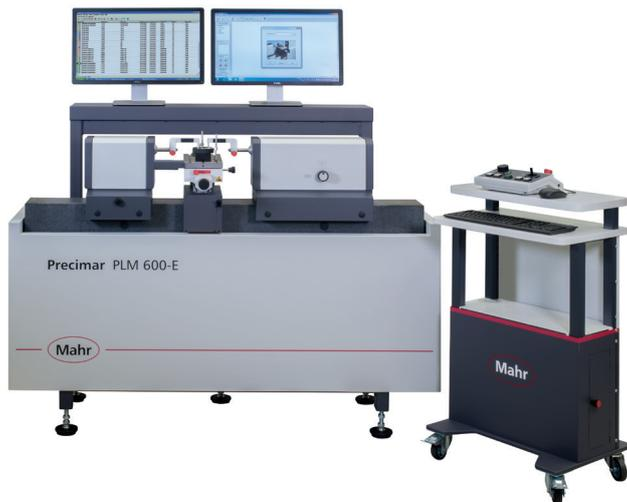
The PLM 600-E precision length measuring machine is an Abbe compliant comparator mounted on highly homogeneous rigid granite in a horizontal configuration
