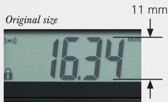
The high-contrast display with 11 mm sized digits enables accurate, fatigue-free reading of the measurement results.
