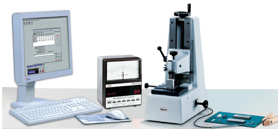
The 826 PC gage block measuring instrument is quick, reliable and highly accurate. An open and extremely rigid L-shaped stand forms the base for the two counteracting precision measuring probes and the absolutely level measuring table.
