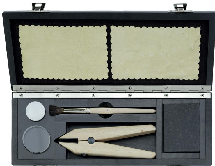
The main tools for testing and repairing parallel gage blocks
