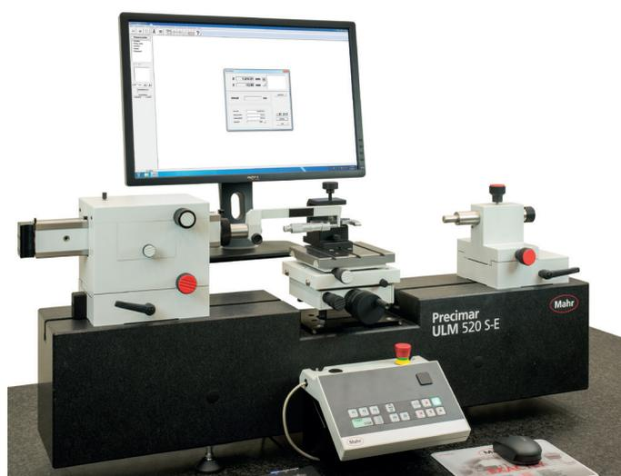
Large universal length measuring instruments with large direct measuring range are mounted on highly homogeneous rigid granite in a horizontal configuration.
