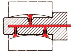
Diameter measurement of cylindrical blind bores with lever contact plug gage.
