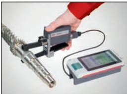
▲ Traverse Drive for Shaft Measurements
